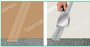
**E. Spread Mortar onto DemoFlex Immediately**
