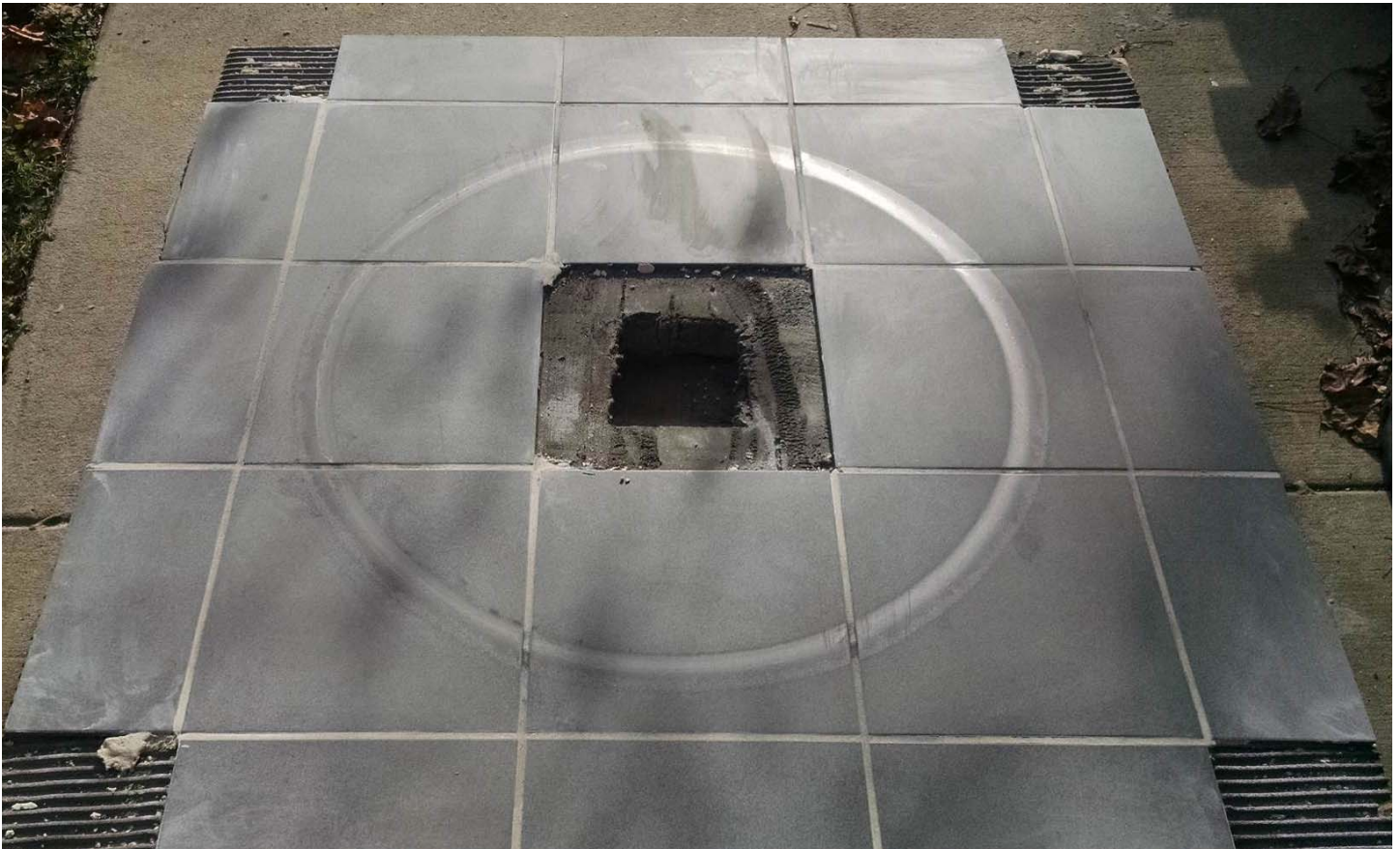
Image 1: Full Assembly showing 12" x 12" Crossville porcelain tiles after testing
